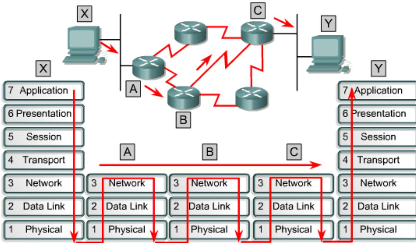
Each router provides its services to support upper-layer functions.
