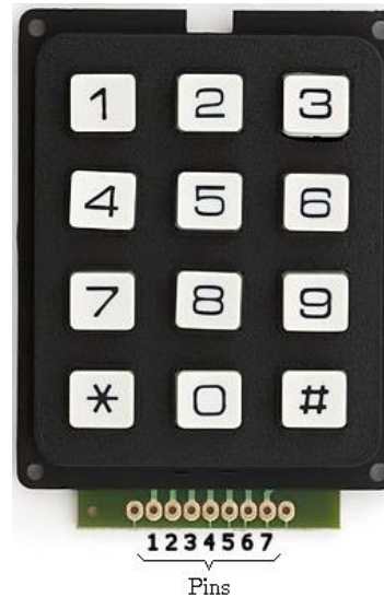
Figure 1: Matrix Keypad Connections
