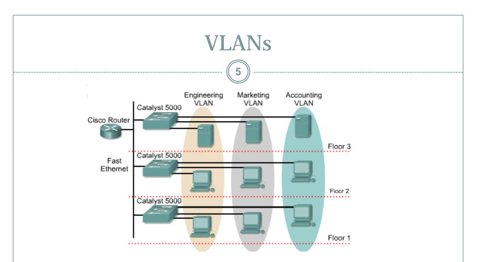
VLANs logically segment switched networks based on an organization's functions, project teams, or applications as opposed to a physical or geographical basis.
