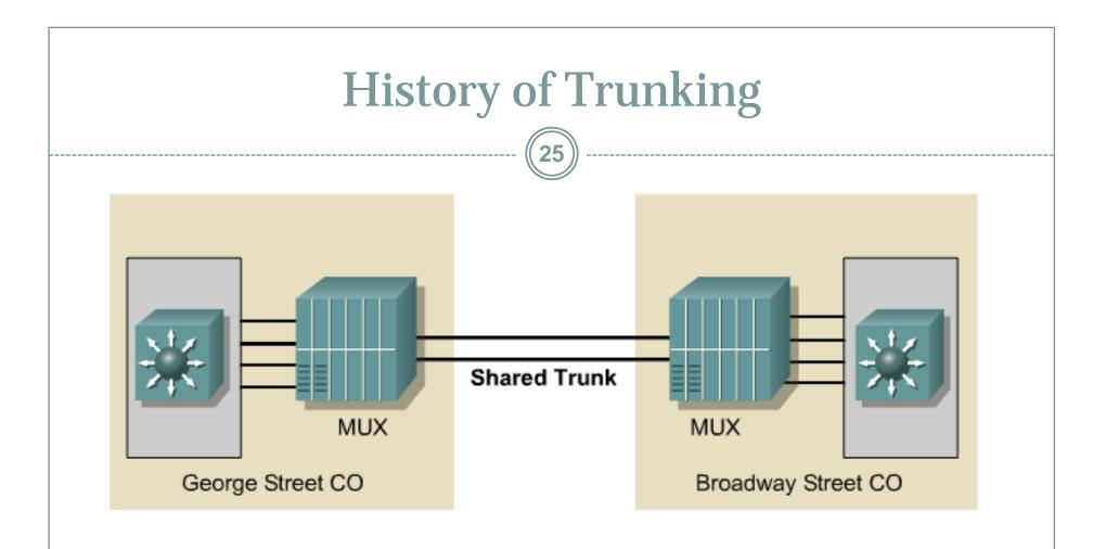
The telephone industry used multiplexers to carry multiple voice signals on a single trunk between COs.
