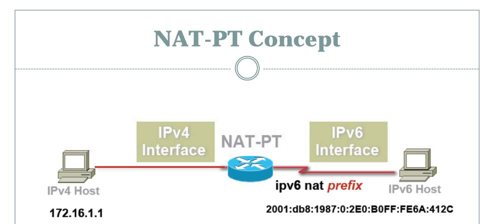
prefix is a 96-bit field that allows routing back to the NAT-PT device
