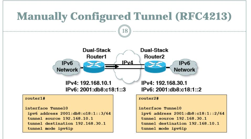
Manually Configured tunnels require: Dual stack end points Both IPv4 and IPv6 addresses configured at each end
