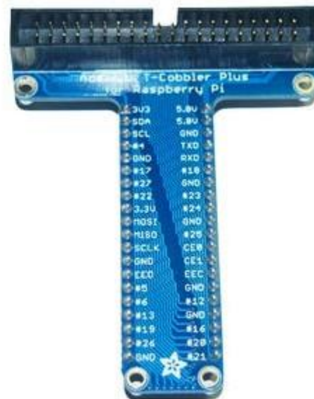
The labels on the various pins on the Adafruit Pi T-Cobbler Plus
