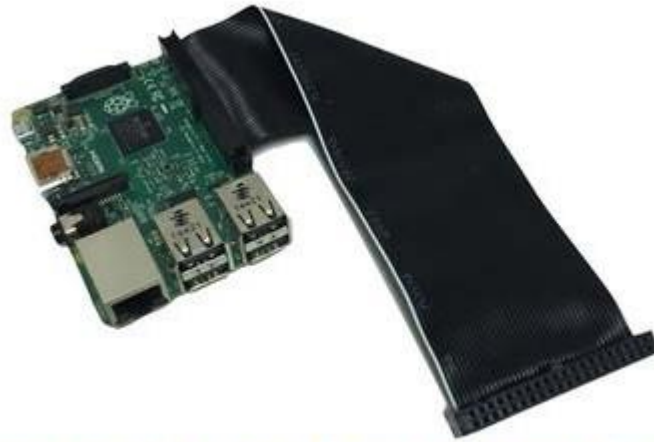
Connecting the Adafruit Pi T-Cobbler Plus to the Raspberry Pi
