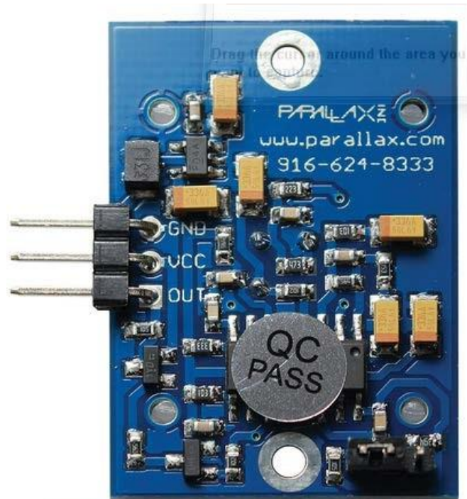
The layout of the various pins on the PIR Motion Sensor
